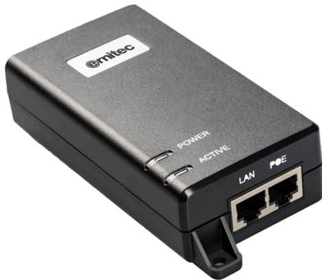
ELECTRA-P2-60W Is a single port PoE Injector. It provides 55Vdc, 1.1A power for remote PDs over full 4pairs output. It supports 10/100/1000Mbps of data speed. It works for 60W PoE PDs, such as wireless APs, Network cameras, IP Phones and other high power Ethernet terminals. It fully complies to IEEE802.3af/at, PoE++ standard.
